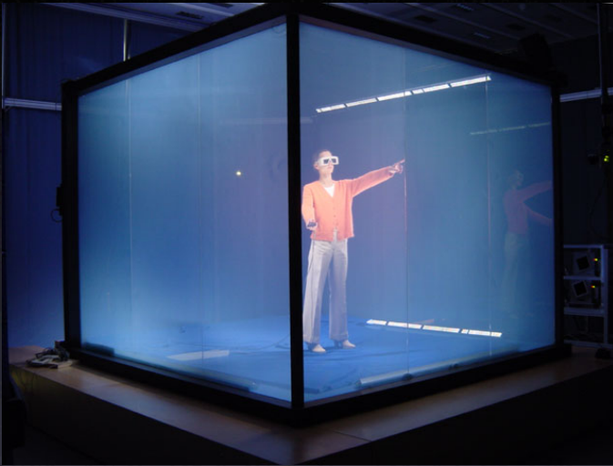
CAVE made of giant shutters so camera array can see in
